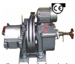
Laboratory Pulveriser is a disc type grinder, designed to grind virtually any material to produce a fine mesh sample in one operation. The instrument is useful for assaying, mining and for metallurgical, quarrying, aggregate processing, chemical, geological and industrial laboratories. It is a self contained grinder, with a rotary disc, having a planetary movement in a vertical plane. This feature gives added life to the moving parts and produces a sample of uniform
